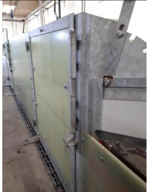
**Figure 5.** This handle can be operated with one hand and the gate 'shuts tight' (Jyden).
